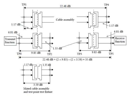
NOTE—The connector insertion loss is 1.07 dB for the mated test fixture. The host connector is allocated 0.62 dB of additional margin.
