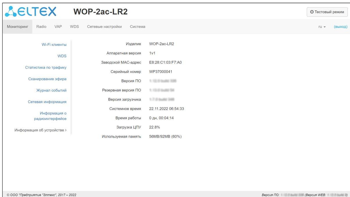
The screenshot shows the 'Information about the device' section of the WOP-2ac-LR2 configuration interface. The left sidebar lists various monitoring and configuration tabs: Мониторинг, Radio, VAP, WDS, Сетевые настройки, Система, and Информация об устройстве >. The main panel displays the following device information:
