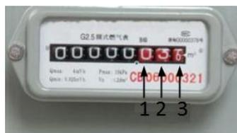
Figure 1 Determining the index of red digit with silver spot
